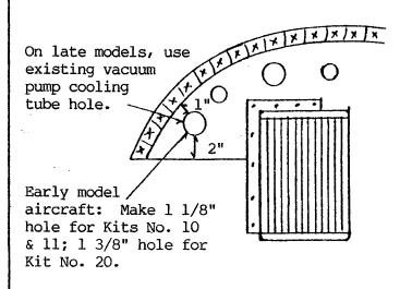
View: L H rear engine baffle, looking forward.
